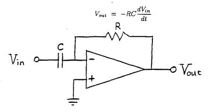
1c. Sketch the output waveform if the input were a symmetrical triangle wave.
