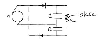
The two capacitors have the same value. The input AC voltage is  $V_I = 141 \sin(377t)$ .
