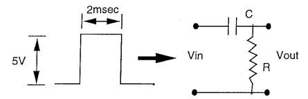
Draw the expected shape of the output pulse (Vout ) below the input waveform (vin) on the attached graph paper and provide calculations to support your answer for the following two sets of values of C and R:
