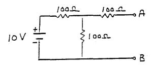
(b) What value of resistance should one connect between terminals A and B in order that the power dissipated in the resistance be a maximum? Justify your answer.
