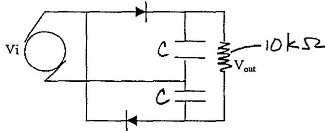
The two capacitors have the same value. The input AC voltage is  $V_i = 141\sin(377t)$ .
