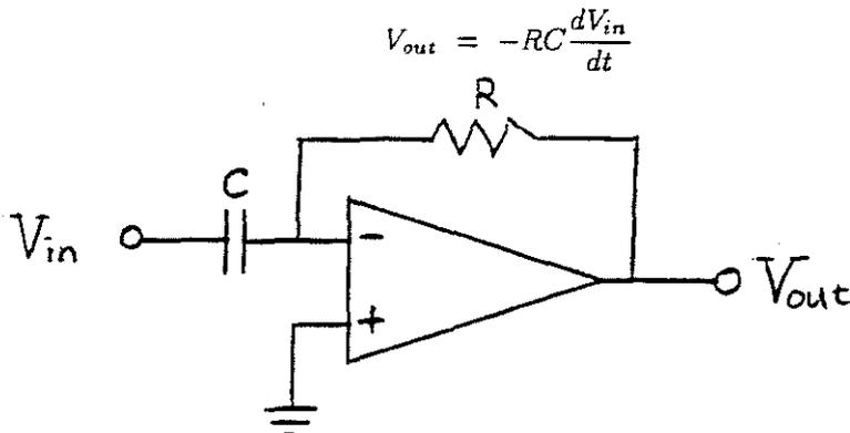
1c. Sketch the output waveform if the input were a symmetrical triangle wave.
