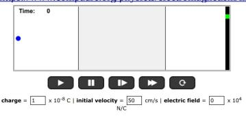
The simulation displays a region where a uniform electric field can be created. When the play button is pressed a charged particle will be released with a specified velocity. You have 3 boxes where you can change the charge on the particle, the initial velocity and the electric field strength.
