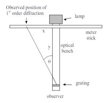
The relationship between the wavelength, the grating spacing and the diffraction angle is
