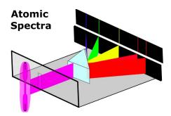
On the left there is a lamp containing He gas. The light emitted from the lamp passes through a prism which disperses the wavelengths at different locations on a screen. The spectra lines are the lines you see on the screen.
