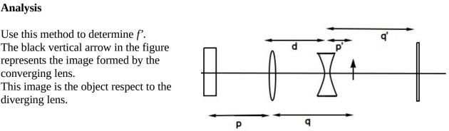
**21.** Measure *p* and use *f* of the converging lens and the equation (1) to calculate *q*
