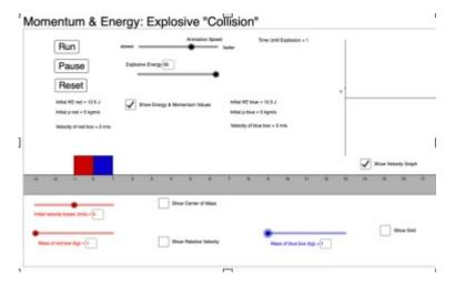
This simulation shows a very simple case of explosion where the initial object, made of both boxes together, explodes into the two separated boxes. The explosion takes place in one dimension. Uncheck the box 'show relative velocity' and 'show center of mass'. Mass of the blue box 2 kg, red box is 2 kg. Change the explosive energy to zero (i.e totally inelastic). Initial velocity of the boxes 3 m/sec. Click *Run* to start the simulation.
